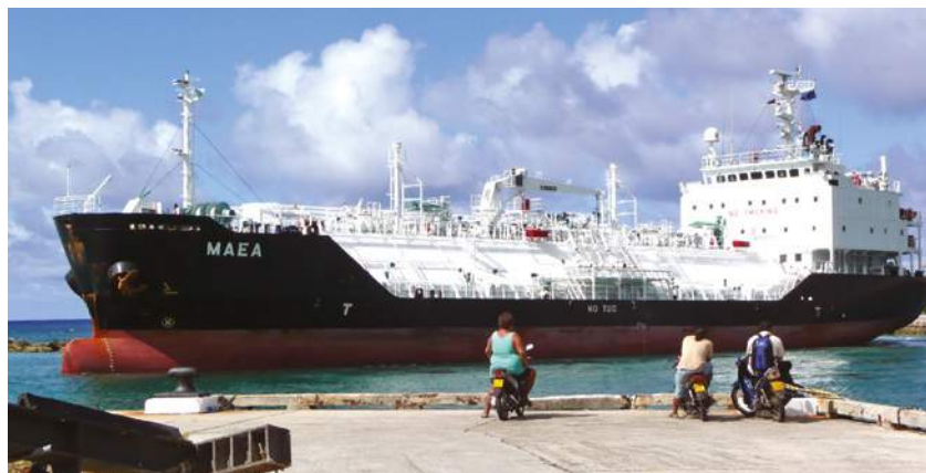
The fully pressurised LPGC remains the workhorse of the gas carrier fleet, extending the supply chain into the remotest parts
